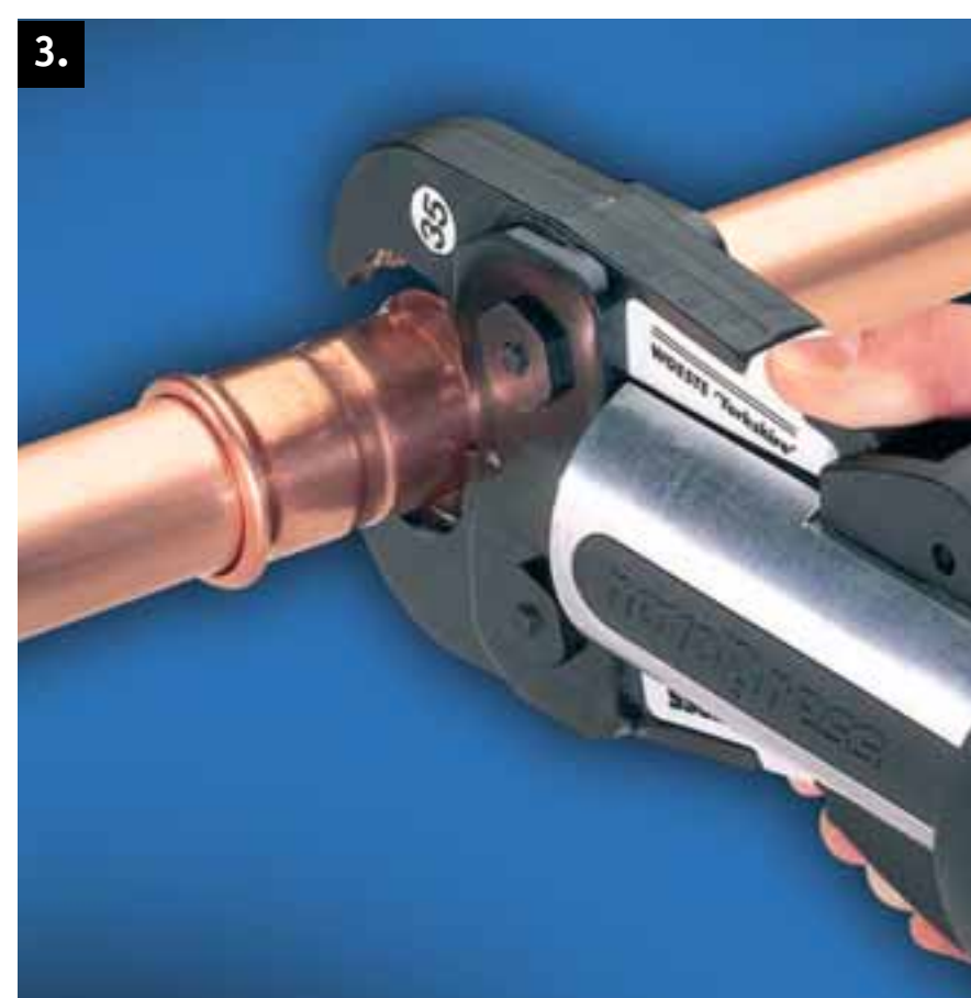
3. Insert the correctly sized jaws into the press-fit tool and place them over the bead at the mouth of the fitting.
