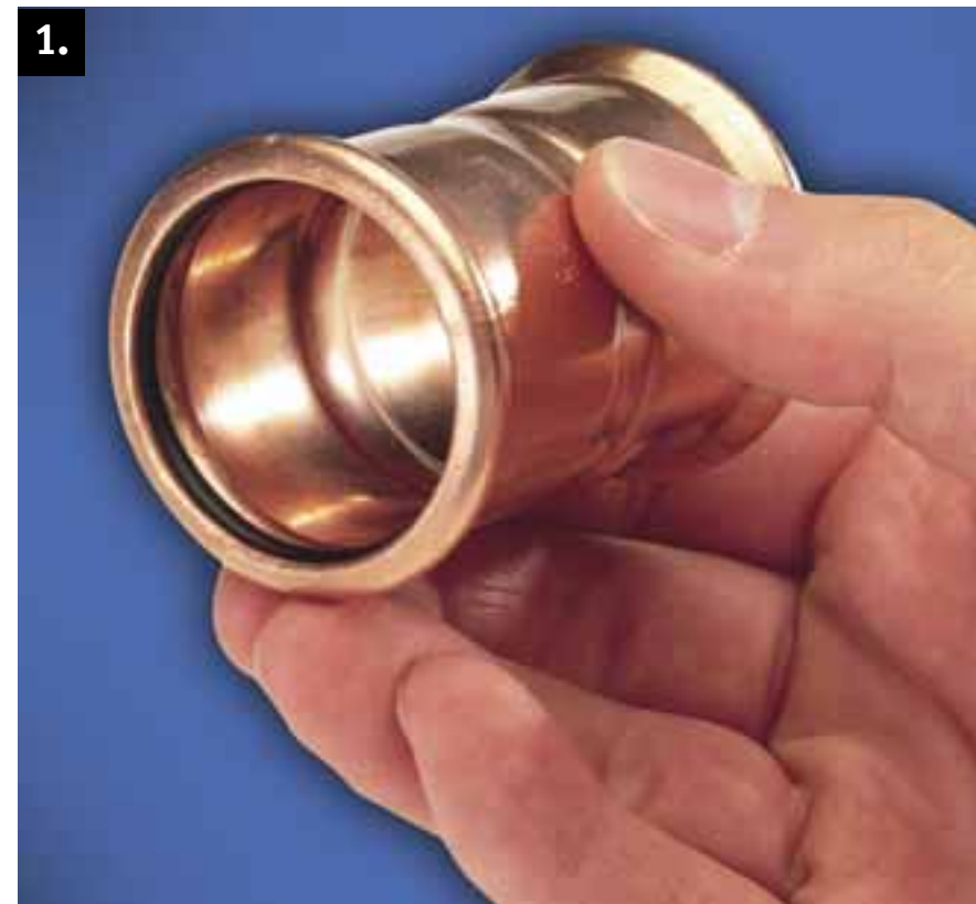
1. Keep all fittings in their bag prior to installation to ensure the lubrication does not dry out. Ensure the 'O' ring is seated correctly within the fitting socket.
