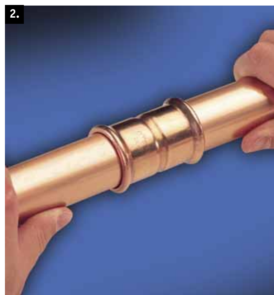
2. Assemble the joint, ensuring the tube is inserted into the fitting until it meets the tube stop, using the insertion depth mark as a visual aid. Only when the tube reaches the tube stop should the pressing operation be undertaken.
