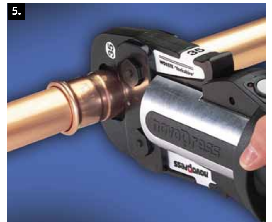
5. Press the trigger or button to start the jointing cycle. When the jaws fully enclose the mouth of the fitting, the joint is complete. The jaw should then be released from around the fitting.
