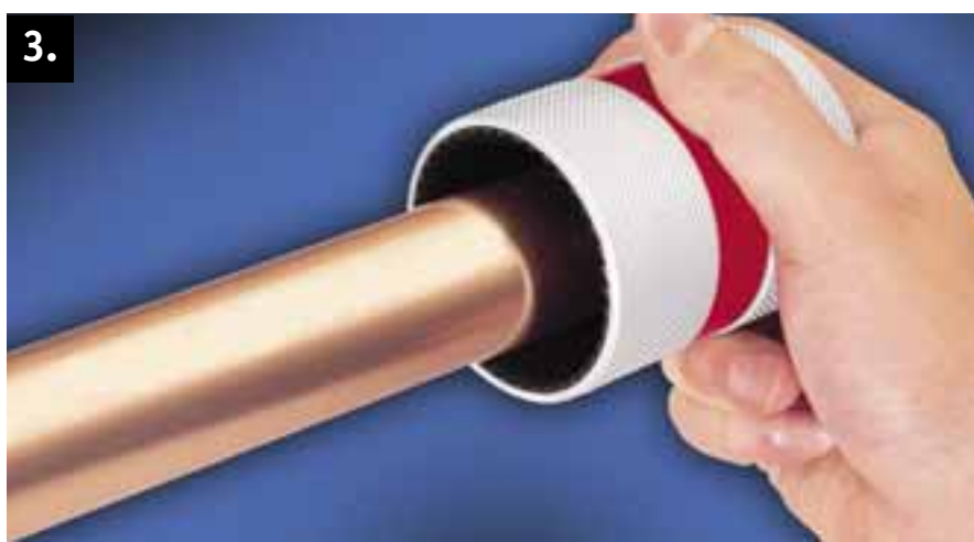
3. Deburr both internal and external tube ends then wipe clean of all swarf and debris to avoid damage to the 'O' ring upon tube insertion. A S120 deburring tool can be used for this purpose.
